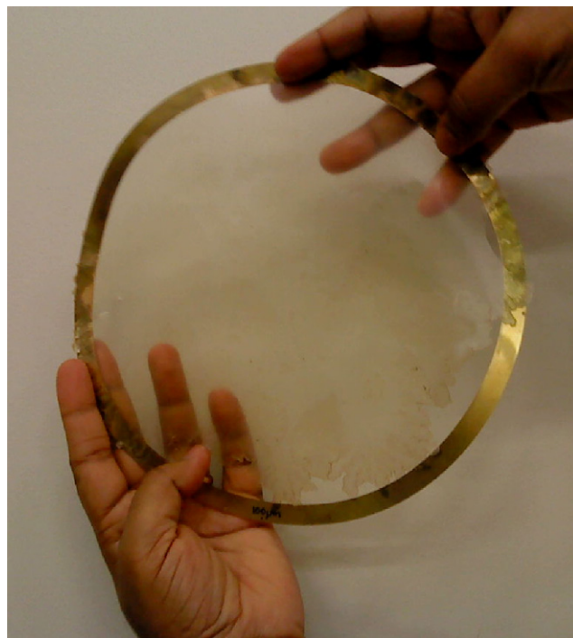
Fig. 9. Hot pressed XG film with 30 wt% sorbitol (0.1 mm thick).
